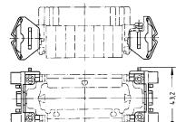
Min. retention force in sheet-metal cut out Mating without guiding system 250 N Mating with guiding system 400 N Unmating without guiding system 400 N Unmating with guiding system 500 N
