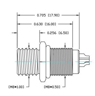
NOTE: MATERIAL HOUSING: PBT UL94V-0, BLACK CONTACT: **BRASS** NUT: BRASS SHELL: BRASS **D-RING**: NBR, BLACK FINISH CONTACT: GOLD PLATED □VER 504 NICKEL SHELL: NICKEL PLATED NUT: NICKEL PLATED **ELECTRICAL** RATED CURRENT: ЗА 60V RATED VOLTAGE: WATER PROOF: IP67 **ENVIRONMENT** OPERATION TEMPERATURE: -40°C TD +85°C
