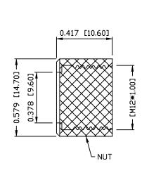
M12 FEMALE - CABLE MOUNT - SOLDER CUP - 4 POS.
