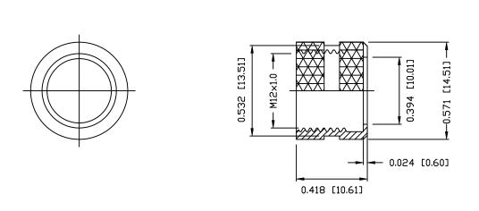
M12 FEMALE - CABLE MOUNT - SOLDER CUP - 4 POS. - D CODE
