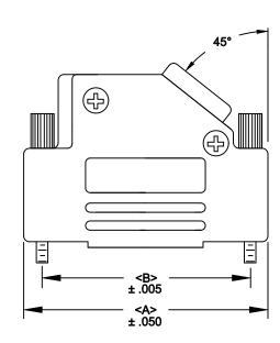
PLASTIC: ABS VH-0800 - NICKEL PLATED - UL 94-HB JACKSCREWS: STEEL
