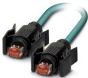
Assembled Ethernet cable, CAT6, shielded, 4-pair, 26 AWG* stranded (7-wire), RAL 5021 (water blue), RJ45 plug/IP67 (black) to RJ45 plug/IP67 (black), line, length: 2 m
