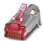
RJ45 male insert, CAT6, 8-pos., shielded, IDC pierce connection, for AWG 27 litz wires ... 24, with strain relief
