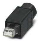
RJ45 connector, IP65/IP67, with push/pull interlocking (version 4), plastic housing, for 10 Gbps, for 24 ... 28 AWG stranded conductors
