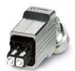
Push-pull connector (version 14), die-cast zinc, with SC-RJ insert for GOF, for cable diameter of 5.5 mm ... 10 mm, cable outlet at the bottom, 10 pcs.
