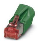
RJ45 connector, Degree of protection: IP20, Number of positions: 8, 1 Gbps, CAT6, Material: PA, Connection method: IDC connection technology, Connection cross section: AWG 24-27, Cable exit: straight
