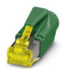
RJ45 connector, Degree of protection: IP20, Number of positions: 8, 10 Gbps, CAT6<sub>A</sub>, Material: PA, Connection method: IDC connection technology, Connection cross section: AWG 24-27, Cable exit: straight
