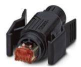
RJ45 connector, Degree of protection: IP67, Number of positions: 8, 1 Gbps, CAT6, Material: PA, Connection method: Crimp connection, Connection cross section: AWG 24-27, Cable exit: straight
