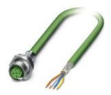
Assembled PROFINET cable, CAT5e, shielded, star quad, AWG 22 stranded (19-wire), RAL 6018 (yellow green), free cable end to M12 flush-type socket, rear/screw mounting with M16 thread, line, length: 2 m
