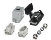
Connector set, Number of positions: 16, Material: Die-cast aluminum, salt water resistant, Connection method: Push-in connection, Connection cross section: AWG 26-14
