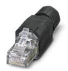
RJ45 connector, IP20, CAT5e, 8-pos., with QUICKON fast connection technology; with packaging for end customers; for 26 ... 23 AWG 1-wire and 7-wire conductors, for a cable diameter of 4.5 mm ... 8.0 mm, marking TIA 568 B, color: black
