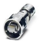
RJ45 connector, Degree of protection: IP67, Number of positions: 8, CAT5 (IEC 11801:2002), Material: Zinc die-cast, Connection method: IDC connection, Connection cross section: AWG 27-24
