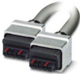
Cable, PROFINET/power, 5-position, PVC, silver-gray RAL 7001, Plug straight MSTB Push Pull / IP65, on Plug straight MSTB Push Pull / IP65, Cable length: 1 m
