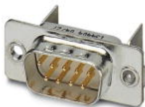
D-SUB contact insert, shell size 1, with nine signal contacts, type of contact pin, for PCB assembly, angled, fixing with a 2.5 mm hole and solder metal plate, for panel mounting frame VS-09-...
