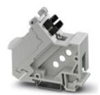
Patch panel, SC-RJ, DIN rail mounting, IP20, 1 slot, socket/socket, can be used for glass, multi-mode, PCF, and polymer fibers
