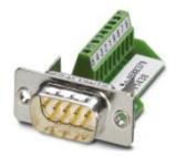
D-SUB contact insert, shell size 1, with 9 signal contacts, male type of contact, screw connection, straight, for panel mounting frame and sleeve housing with IP67 protection
