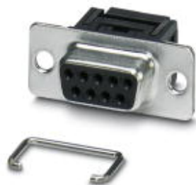
D-SUB contact insert, shell size 1, with nine signal contacts, type of contact socket, flat-ribbon cable connection, angled, fixing with a 3 mm hole, for panel mounting frame VS-09-...
