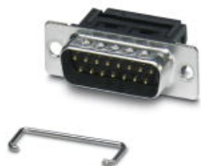
D-SUB contact insert, shell size 2, with 15 signal contacts, type of contact pin, flat-ribbon cable connection, angled, fixing with a 3 mm hole, for panel mounting frame VS-15-...
