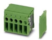
PCB terminal block, Nominal current: 32 A, Nom. voltage: 320 V, Pitch: 6.35 mm, Number of positions: 10, Connection method: Front screw connection, Mounting: Wave soldering, Conductor/PCB connection direction: 0 °, Color: green
