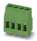
PCB terminal block, Nominal current: 24 A, Nom. voltage: 400 V, Pitch: 5.08 mm, Number of positions: 2, Connection method: Screw connection with tension sleeve, Mounting: Wave soldering, Conductor/PCB connection direction: 0 °, Color: green, The article can be aligned to create different nos. of positions!
