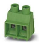
PCB terminal block, Nominal current: 32 A, Nom. voltage: 1000 V, Connection method: Screw connection with tension sleeve, Mounting: Wave soldering, Conductor/PCB connection direction: 0 $^{\circ}$ , Color: green
