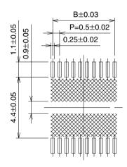
Note: Shaded area should be free of any conductive traces.
