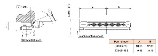
Notes The maximum opening angle of the rotating mating/unmating guide is 25°. Do not exceed this angle.
