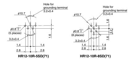
Remarks: Dimensional tolerance of  $\pm 0.05$ mm is recommended for the board arrangement.
