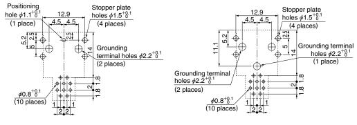
Remarks: Dimensional tolerance of  $\pm 0.05$ mm is recommended for the board arrangement.
