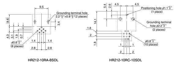
Remarks: Dimensional tolerance of  $\pm 0.05 \text{mm}$  is recommended for the board arrangement.
