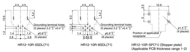
Remarks: Dimensional tolerance of  $\pm$  0.05mm is recommended for the board arrangement.
