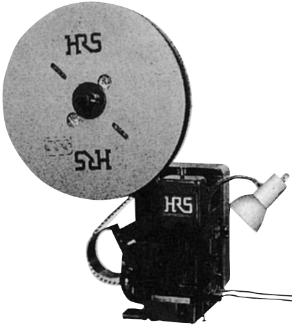
Automatic crimping press (CM-105)
