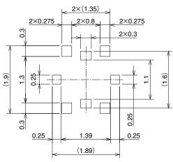
: This area must be free of conductive traces and resist field.
